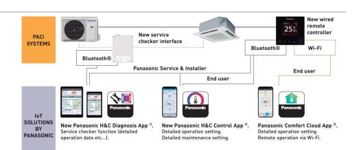
A service checker interface is required when this app is used from outdoor location. Wired remote controller (CZ-RTC6BL or CZ-RTC6BLW) is required when this app is used from indoor location. Available from winter 2020, compatible with PZ3 and PZH3 outdoor units. 2] CZ-RTC6BL or CZ-RTC6BLW required. 3] CZ-RTC6BLW required.
